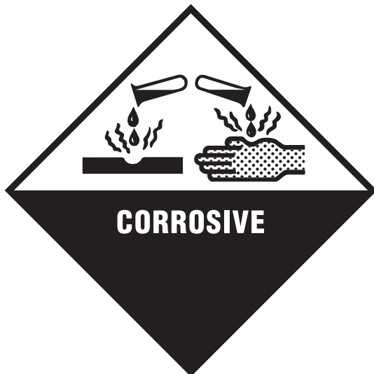
corrosive subsidiary risk label
